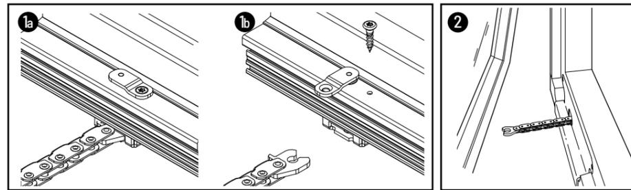
2. To reconnect the chain, power the chain out to meet the sash.
