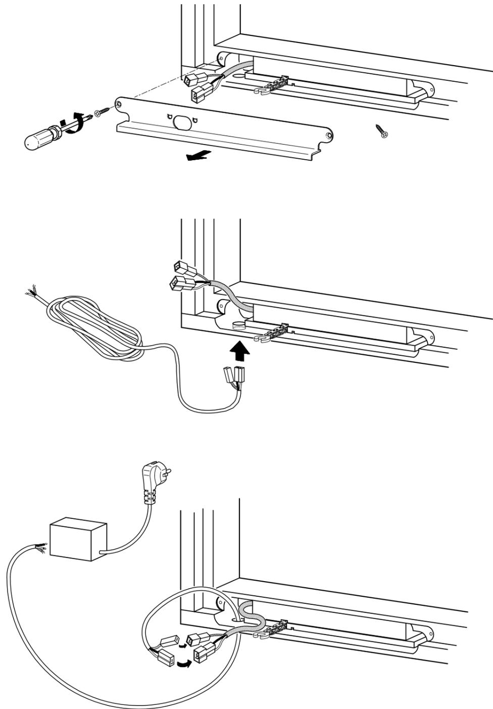
1. First open the window, then disconnect the chain (4x20 US screw):
